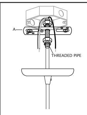
11. Slightly loosen ground screw on mounting bracket (A). Do not completely remove ground screw. Wrap house ground wire (copper) around ground screw, leaving enough ground wire to attach to fixture ground wire. Twist end of fixture ground wire and end of house ground wire (copper) together. Twist wire nut (C) onto ends of wires. Completely tighten wire nut (C). Reference chart below for correct wiring instructions.
