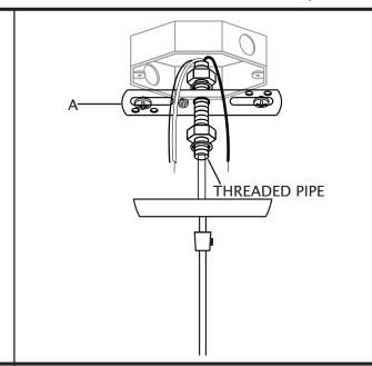
10. Slightly loosen ground screw on mounting bracket (A). Do not completely remove ground screw. Wrap house ground wire (copper) around ground screw, leaving enough ground wire to attach to fixture ground wire. Twist end of fixture ground wire and end of house ground wire (copper) together. Twist wire connector (C) onto ends of wires. Completely tighten wire connector (C). Reference chart below for correct wire connections.
